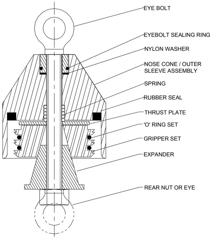
This newly developed Towing Head (Pipe Puller) has been designed specifically for use in Directional Drilling. Providing a cost effective Towing Head which prevents the ingress of drilling fluids into the pipe, whilst being suitable for both SDR 11 and SDR 17.6 pipe (and any SDR in between). Grippers are also available for pipes in the SDR range 21 to 33.
